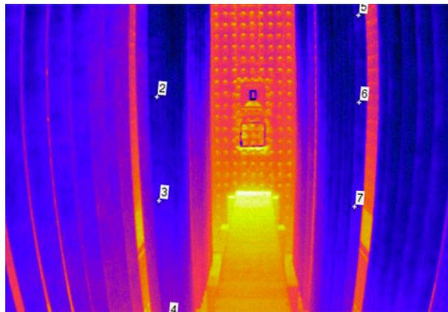
Figure 2. Thermal View inside and Reformer Tube Furnace with data points.
