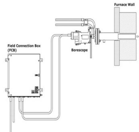
Figure 1. The Thermal imaging cameras are inserted into the reformer, with the end of the imager ¼" from the inside reformer wall refractory. Imagers are water and air-cooled, ensuring accuracy in the hot atmosphere of the reformer. Source: AMETEK Land
