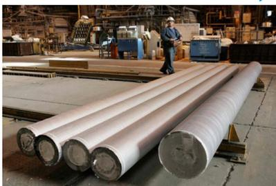
Figure 1. Extrusions begin with aluminium billets. Source: AMETEK Land
