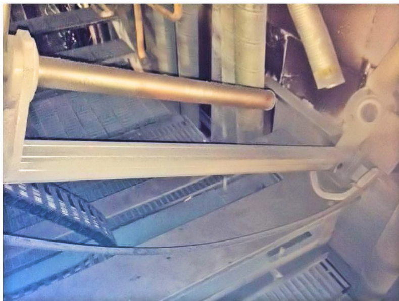
Figure 5. NIR-b on auto retraction mechanism – shown retracted
